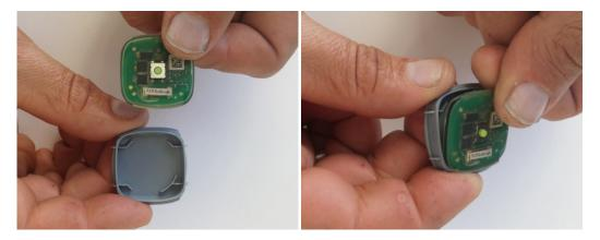
Place the circuit board into the bottom shell as pictured. Use position of data matrix label as reference for how to turn the circuit board.
