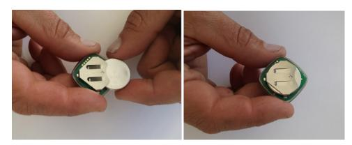
Put the new battery in the battery holder. Check the battery polarity and position the battery accordingly.
