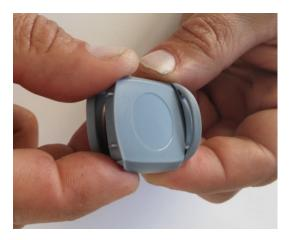
Assemble the Bottom shell with the circuit board in a new Top shell by first placing one of the edges with the snaps in the top shell
