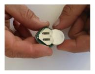
Remove the battery. Dispose of the battery according to the local instructions for recycling, see section "Eliminación".
