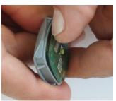
There is a heel protruding on 2 sides from the circuit board. Use fingernail or a small flathead screwdriver gently on this heel to remove the circuit board from the bottom shell. Be careful not to damage the circuit board.
