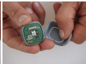
Push the loops outwards with the thumbs until the bottom pops out. Discard the top shell.
