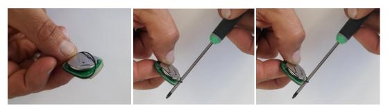
Place the new O-ring in the groove. Make sure it is not twisted.
