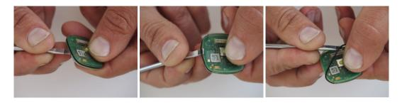
Use a thin flathead screwdriver to remove the O-ring. Be careful not to damage the O-ring groove.
